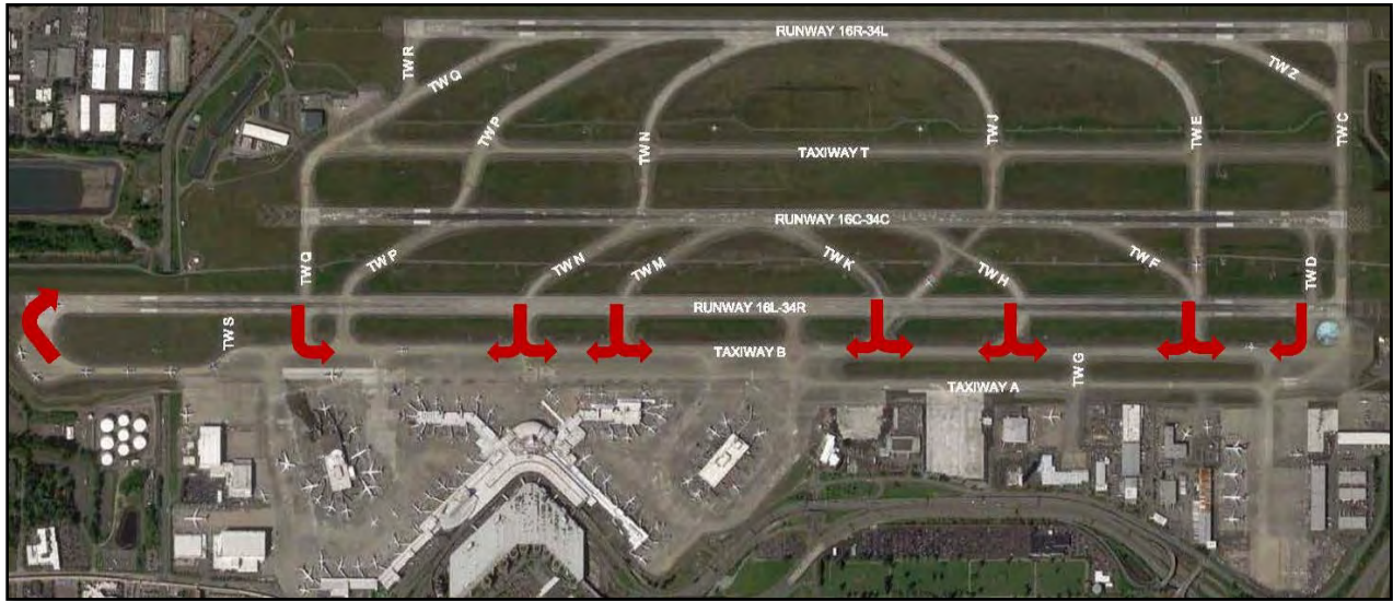
Figure 2-6 Taxiway Intersections Where Fillet Widening is Required to Meet Standards for Boeing 777-300 Turning Movements Seattle-Tacoma International Airport
